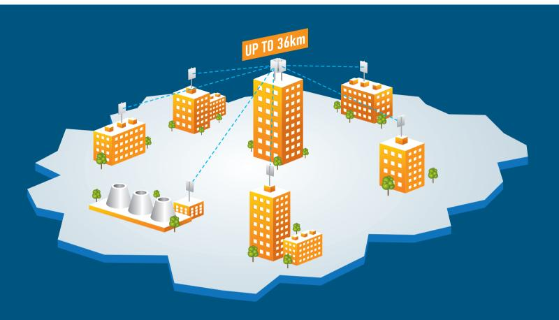
Our family of Point-to-Multipoint solutions are also available in frequency bands from 2.3 to 6.4 GHz and are based on innovative high-capacity base stations and subscriber terminals, reaching up to 240 Mbps and 100 Mbps respectively.
